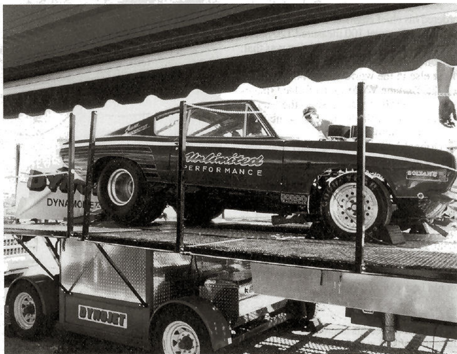
Mobile Dynojet dynos were a natural for racing, allowing teams to check horsepower right at the track.
